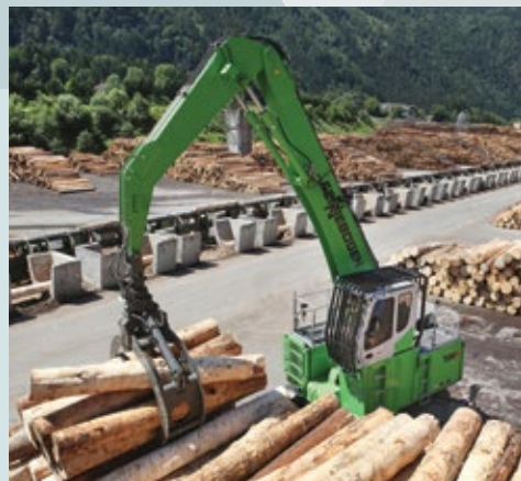
The 360° rotating upper carriage allows a simple manipulation between the rows of stacks
