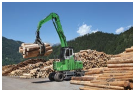
The articulated boom behind the center of the machine enables an optimum weight distribution during transport
